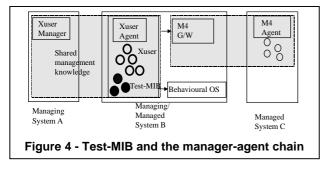
Position of the Test-MIB in the TRUMPET manager-agent chain is shown on Figure 4 (extended from [ii]). Hollow objects represent objects of the Xuser MIB, *i.e.* the information model provided by system B (in our case PNO) to system A (VASP). In practice, some operations performed by system B on the managed objects in its MIB (on behalf of the system A) will involve further operations on the objects in system C,
