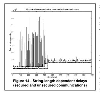
roughly 40%. Before the step increase, the fluctuations around the mean delay value are as drastic as for the fixed-length parameter secured management operation delays discussed in section 4.2. However, after the step increase in the delay, the fluctuations settle down, becoming comparable with the unsecured operations case from Figure 13.
