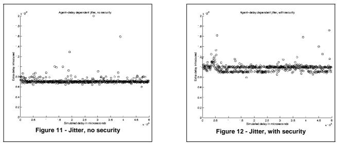
Overall, it can be noted that the agent-simulated delay does not significantly influence the timesensitive performance of the management communications mechanism, both with and without security. In this case, the use of TRUMPET security package does not introduce potential risks to integral operation, when compared to the unsecured operations.
