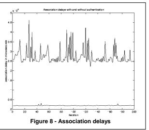
association delays without authentication. It can be seen that the association delays for the secured management association are not just considerably higher, but also that the fluctuations around the mean value are an order of magnitude larger: the secure association establishment introduces an arbitrary delay. This feature of the TRUMPET security package could present a drawback in its use in the time-sensitive applications, where the time constraints are rigorously defined.
