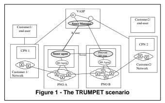
The critical point of the management systems' interconnection is the TMN X interface, such as the Xuser between the VASP and the PNO and the Xcoop between the two PNO OSs. There are two basic requirements on these interfaces: **integrity**, referring to the correct and proper operation of the interconnected management systems and the supporting communications mechanism, in terms of *functionality* and *performance* [iii]; and **security**, referring to the secure and authenticated management
